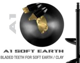
EARTH AUGER FOR GENERAL PURPOSE DRILLING Designed to reduce auger jam, the A1 auger features its cutters on one side as well as a restrictor plate to reduce overrun. Available in earth or tungsten carbide (TC), providing longer wear life and greater cutting performance. Not suited for rock.
